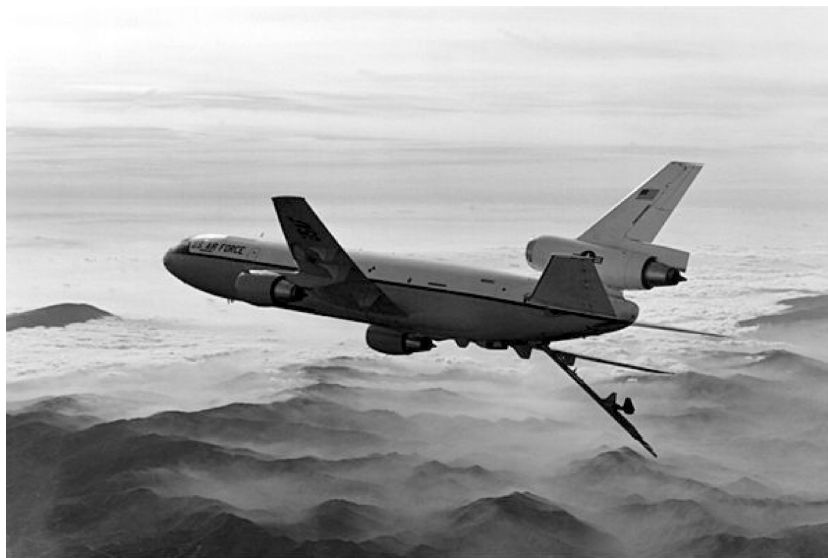
Fig. 10 KC-10A advanced refueling boom (courtesy of The Boeing Company).
