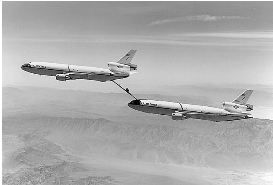
Fig. 1 Wide-body aircraft in-flight refueling (courtesy of The Boeing Company).
